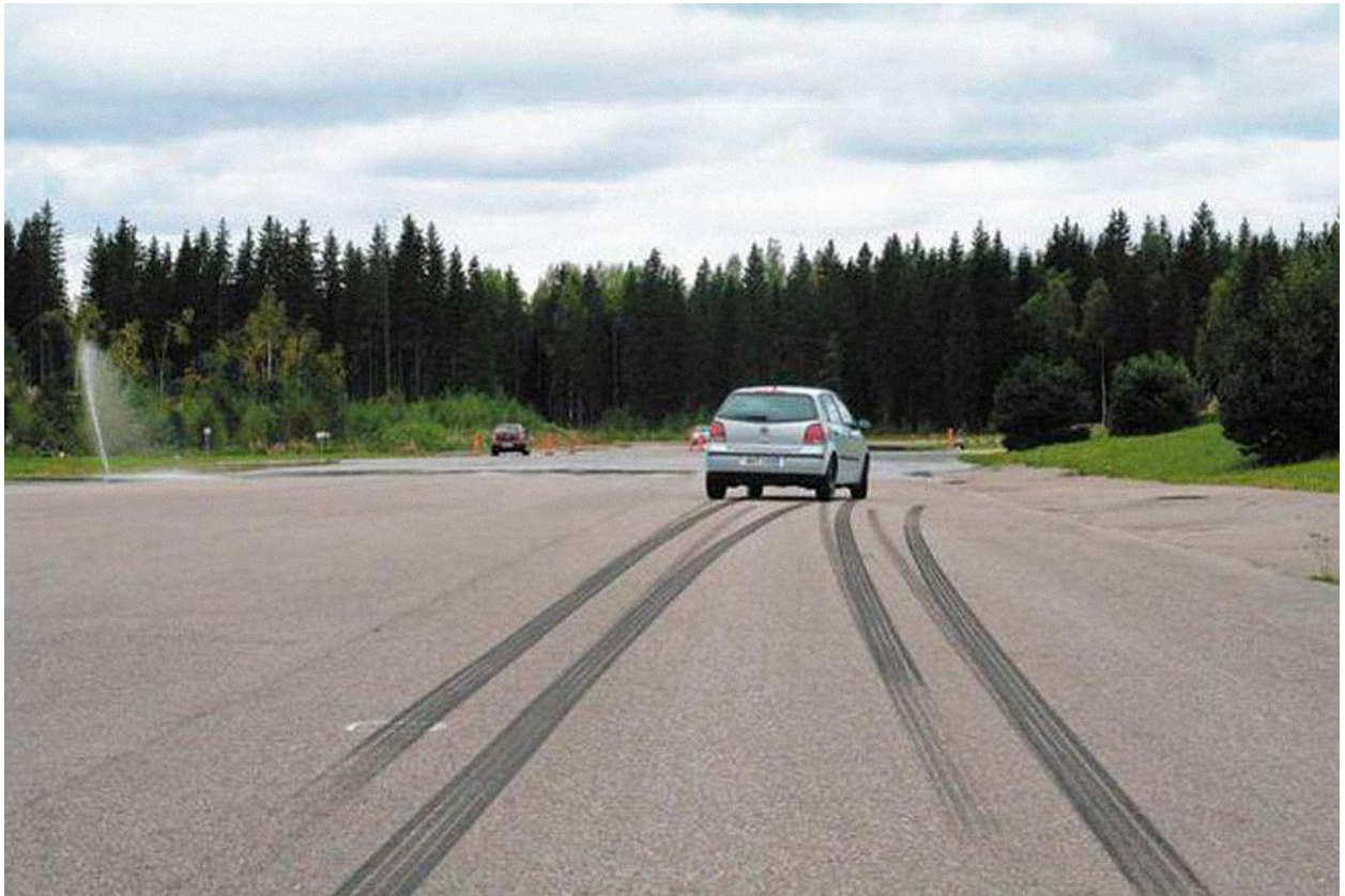
Slika 120: Sledi gum pri zaviranju (vir: https://sl.puntomarinero.com/braking-distance-during-emergency-braking/ , pridobljeno 1. 10. 2019)
